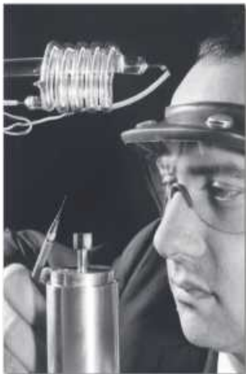
Theodore H. Maiman of Hughes Aircraft Company shows a tube of synthetic ruby crystal, the material at the heart of the first laser. Hughes Aircraft Company
