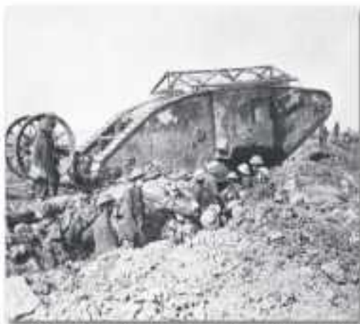
British Mark I tank with anti-aircraft roof and "tail," 1916. Courtesy of the Imperial War Museum, London; photograph, Camera Press
