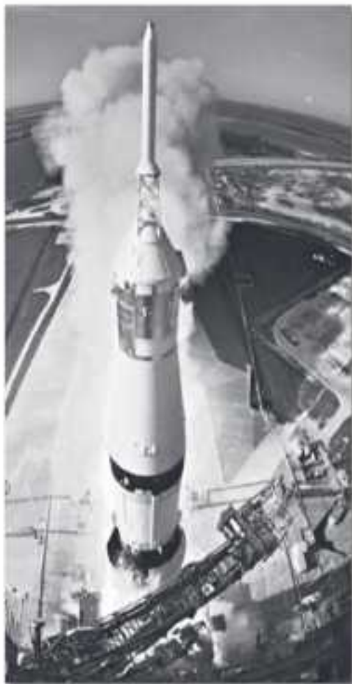
The Apollo 11 spacecraft lifts off from Cape Kennedy, Florida, U.S., atop a Saturn V three-stage rocket, July 16, 1969. A camera mounted at the mobile launch tower's 360-foot (110-m) level recorded this photograph. NASA.
